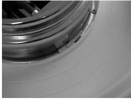
Figure C Metal tab on unit fitted with plastic tab on bowl to Lock and Unlock extractor head
