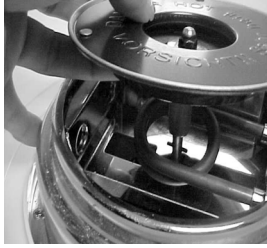
Figure A Removing the Extractor Head Assembly
